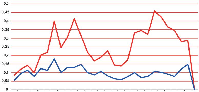
Red line: Acceleration values on the vehicle floor under the hoverboard Blue line: Acceleration values at the plate surface of the hoverboard
