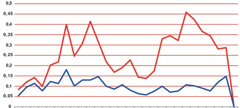
Red line: Acceleration values on the vehicle floor under the hoverboard Blue line: Acceleration values at the plate surface of the hoverboard
