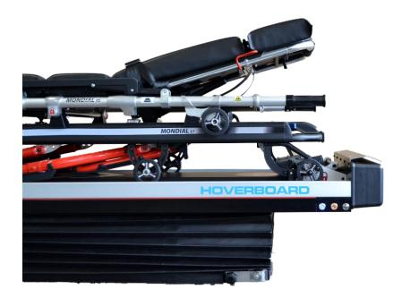
The fully automatic air suspension absorbs most of the incoming vibration energy.
