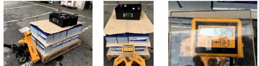
Then we loaded that pallet to the Stryker PowerPro by means of a forklift. Loading is logged on the video „Stryker heavy load test 1635.mov“
