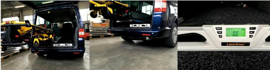
Then we used ramps to situate the vehicle in an angle of 5,8°:
